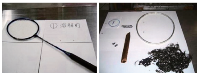
図2 CFRP製バドミントンラケットの溶解処理前(左)と処理後(右) Figure 2 A treated CFRP badminton racket, before (left) and after (right)
