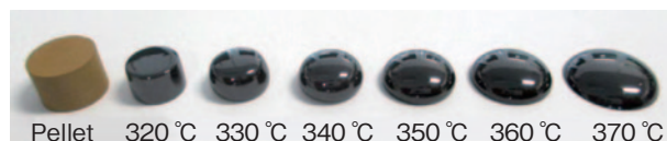
Figure 1 Button Flow Test of Glass Powder
