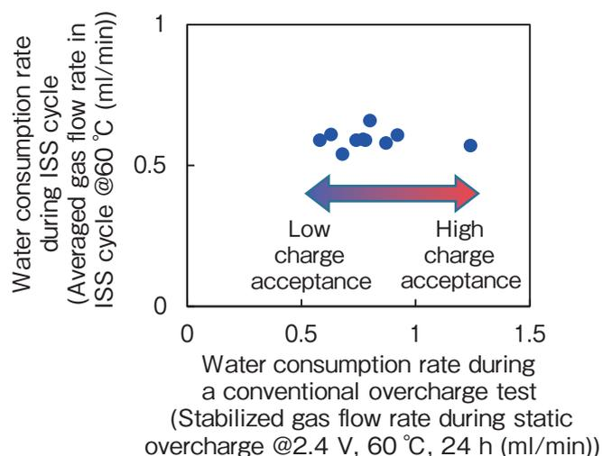
Figure 2 Comparison of water consumption rates during a conventional overcharge test and ISS cycle
