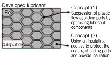
Figure 2 Concept of the developed lubricant
