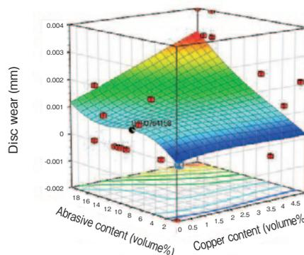
Figure 4 Effect of Copper on the Relationship between Abrasive Volume and Disc Wear
