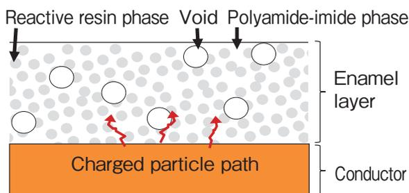
Figure 5 Schematic diagram of cross-section of enameled wire
