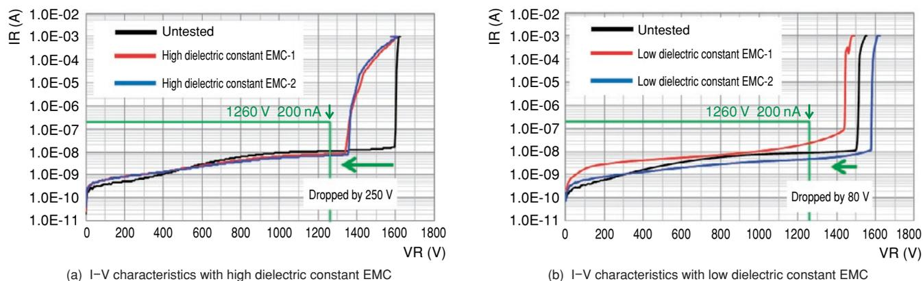
Figure 2 Evaluation result of I-V characteristics with high or low dielectric constant EMC
