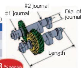
Figure 4 Weight Reduction Effect of Balancer System
