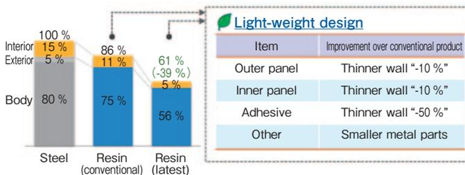
Figure 2 Weight Reduction Effect of Back Door Resinification
