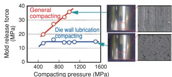
Figure 1 Mold releasability of developed lubricant
