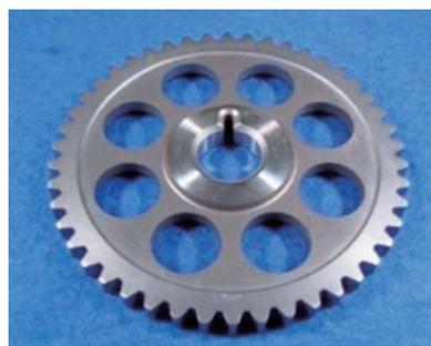
Figure 3 High-density sintered sprocket for silent chain made by die wall lubrication compacting with liquid coating
