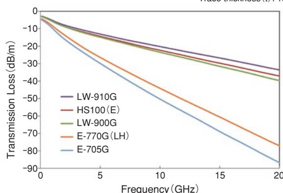
Figure 3 Transmission Loss of MCL-HS100
