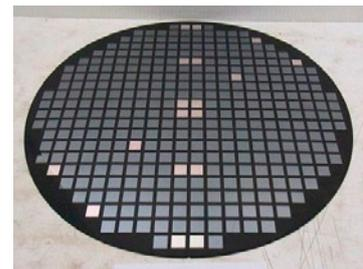
Figure 5 FO-WLP test vehicle made at Open Laboratory
